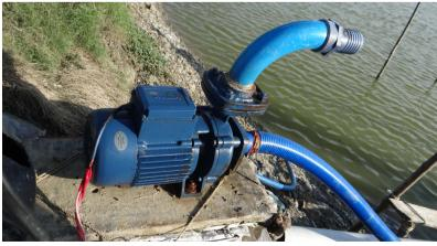
1.5 HP pump for suction and delivery of water into the box cage pipe, controlling flotation and submersion.
