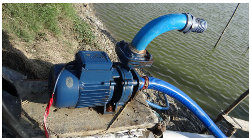
1.5 HP pump for suction and delivery of water into the box cage pipe, controlling flotation and submersion.
