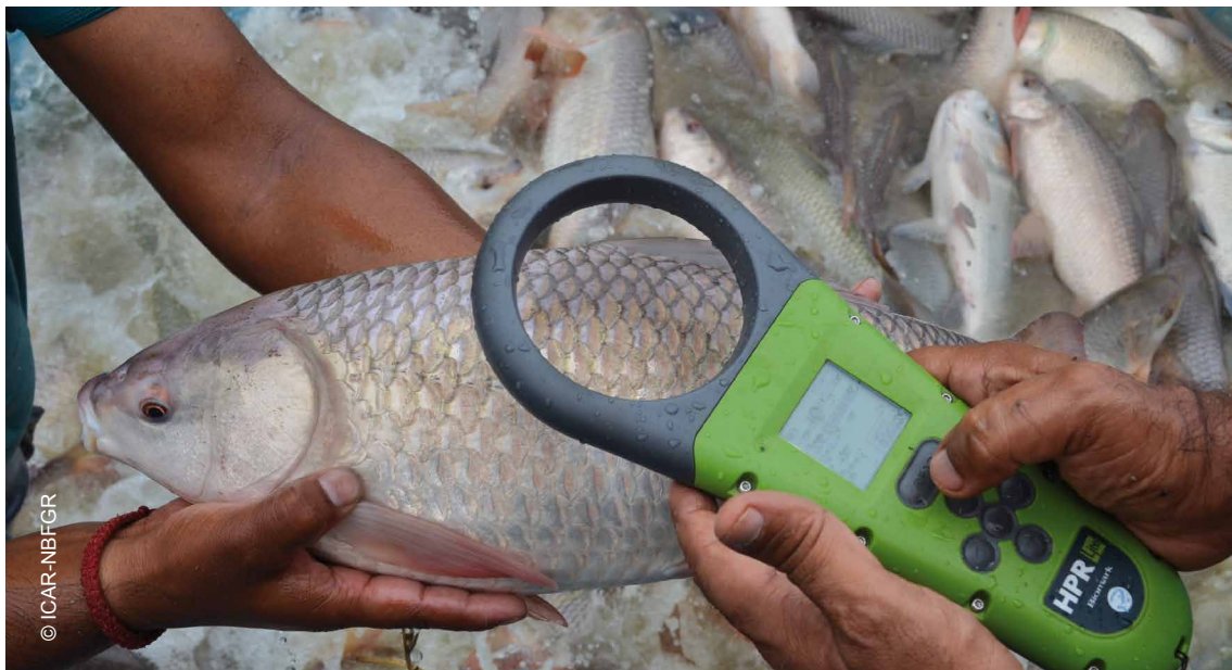
Figure 4. Selection of rohu ( Labeo rohita ) broodstock using PIT tags to identify individual broodstock.
