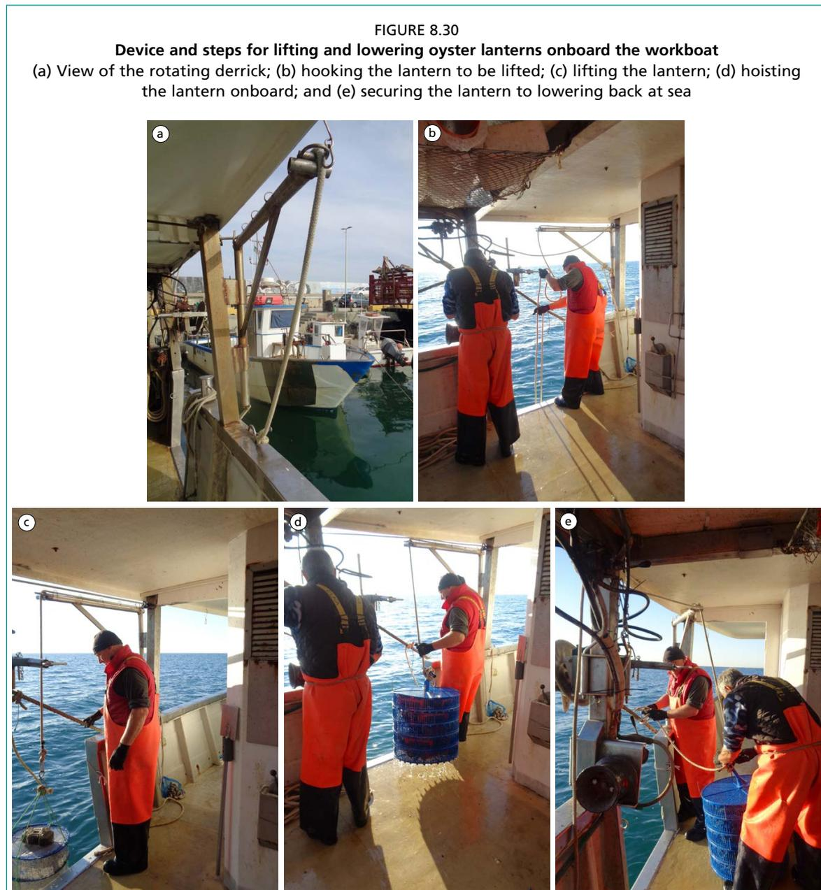
It is important to note that this technical solution imposes a restriction on the use of lanterns exceeding the vertical distance between the deck and the roof. Moreover, the limited width of the opening along the side of the boat increases the difficulty and time involved in the operation, with an increased risk of potential damage to the lanterns.
