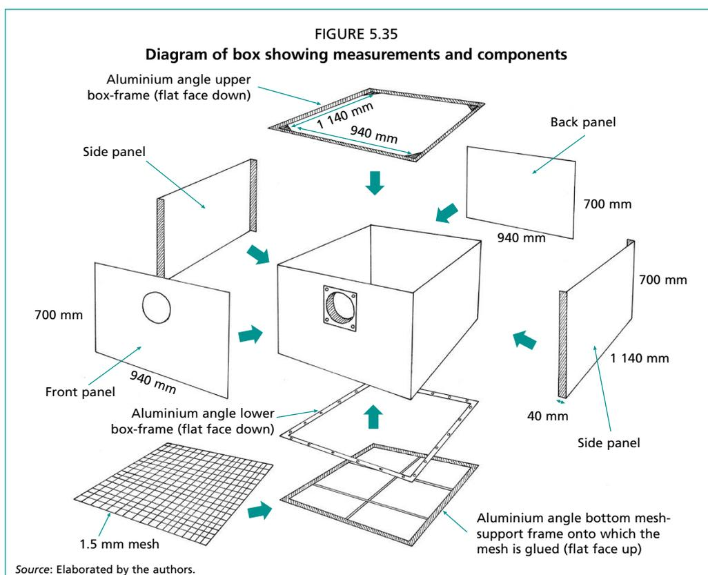
17. Secure the mesh-support frame to the box using 5 × 20 mm bolts and locking nuts.
