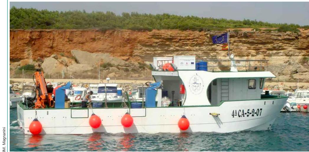
It is also important to note that the use of a crane requires a free and unobstructed area, which may lead to a reduction in deck space and storage capacity for farm equipment and empty lanterns. In the design phase of the workboat, it is crucial to consider the diverse tasks at hand, emphasizing the need for an adaptable deck space. A flat and partly open deck configuration is recommended to facilitate easy customization according to the specific tasks to be accomplished.
