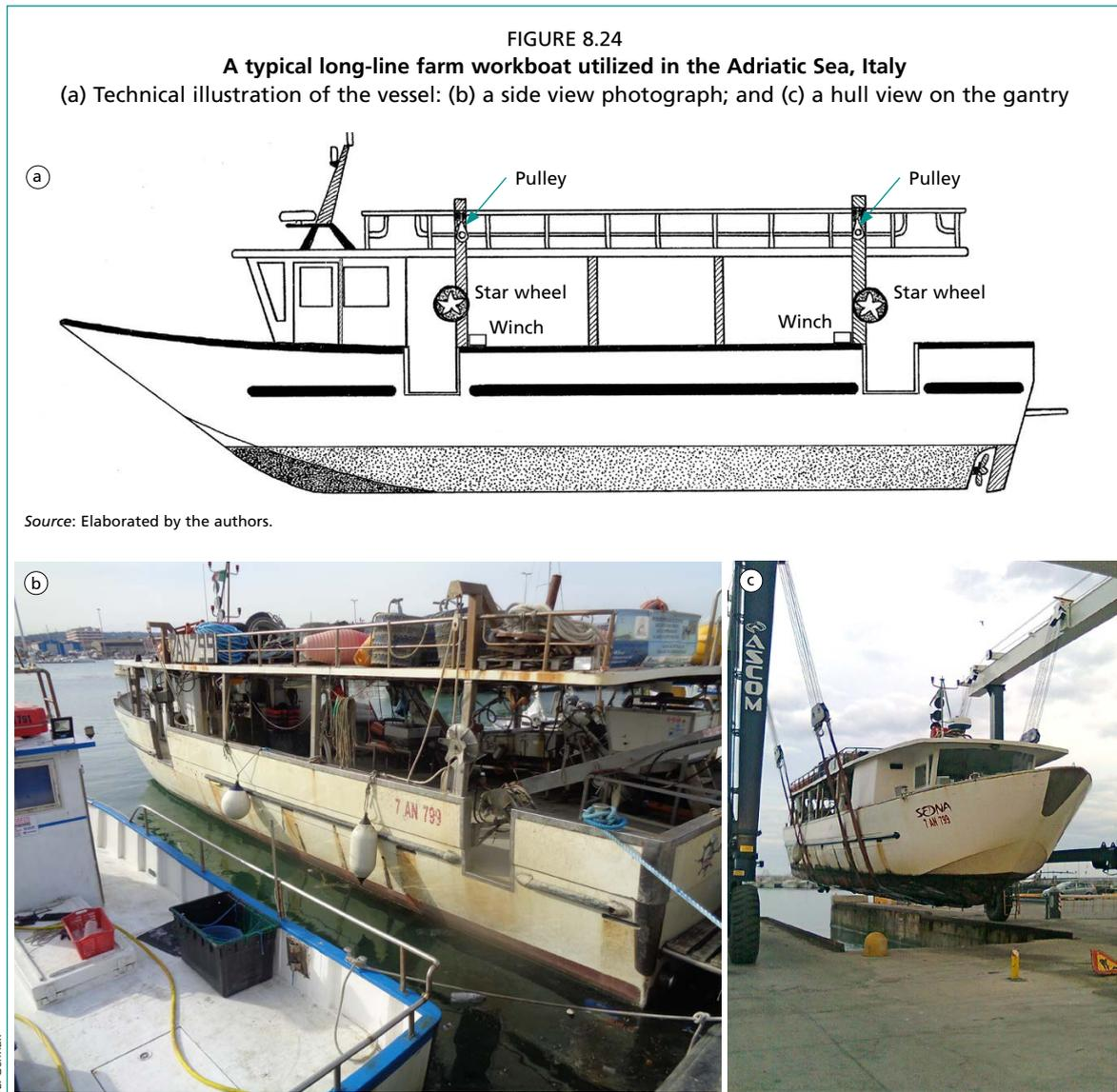
The “V” shaped hull design facilitates rapid navigation, achieving speeds of up to 9 nautical miles per hour, while keeping fuel consumption relatively economical. The vessel’s width of 5.2 m ensures stability during onboard operations and provides ample deck space for equipment installation, product handling, temporary storage, and staff mobility (Figure 8.25).
