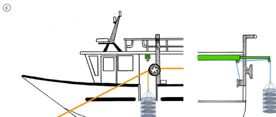
A robust metallic sliding arm paired with a lifting rope, one end of which is equipped with a hook for securing and lifting the lantern, while the other end is wound around the winch.
