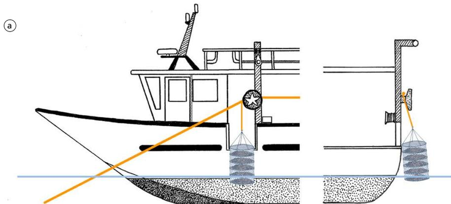
Lifting lanterns with on-board equipment on a traditional mussel vessel requires some adaptation to prevent lantern damage and enhance efficiency. Two additional and improved devices are detailed in (b) and (c) below.
