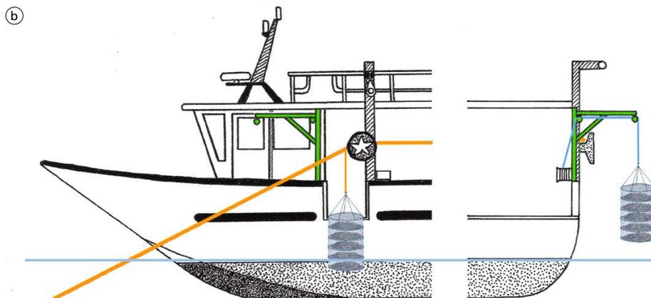
A rotating derrick paired with a lifting rope, one end of which is equipped with a hook for securing and lifting the lantern, while the other end is wound around the winch.
