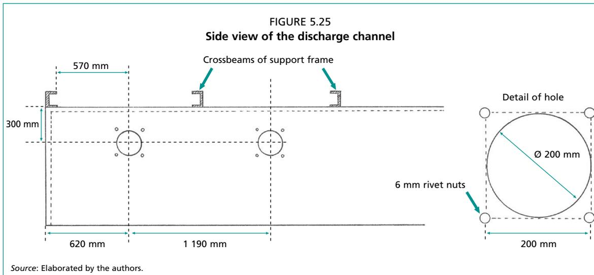
The flanges that are used to connect the seed boxes to the discharge channel are identical to the porthole sock supports that are mounted inside the seed boxes. Please reference page 111 and Figures 5.36c and 5.36d for further details. These should be attached using 20 × 6 mm stainless steel bolts to the exterior of the discharge channel around the pre-cut 200 mm holes shown in Figure 5.25. There are 10 units in total.
