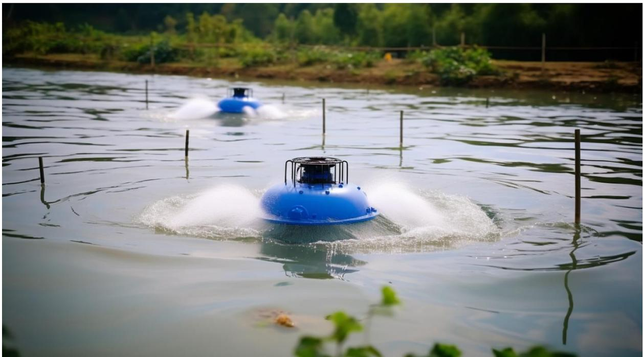
**Figure 116. Propeller-type aerator.**
