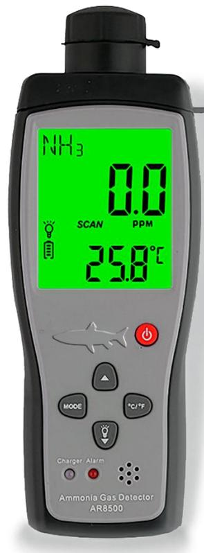
**Figure 53. Ammonia meter. The device already provides results in mg/L of NH<sub>3</sub>.**
