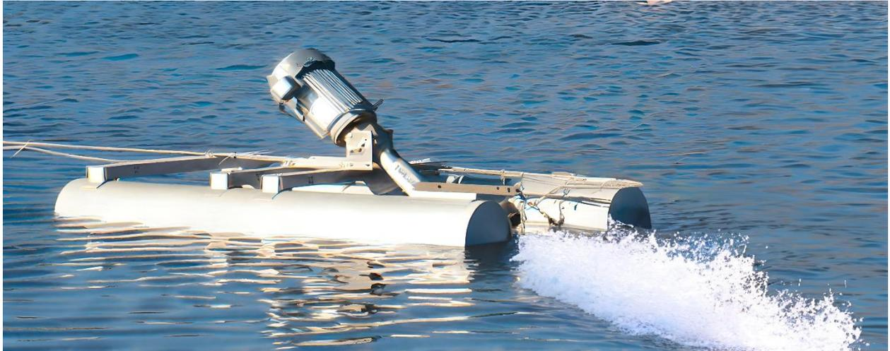
**Figure 115. Impeller aerator.**
