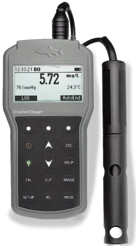
Figure 43. Electronic dissolved oxygen meter.
