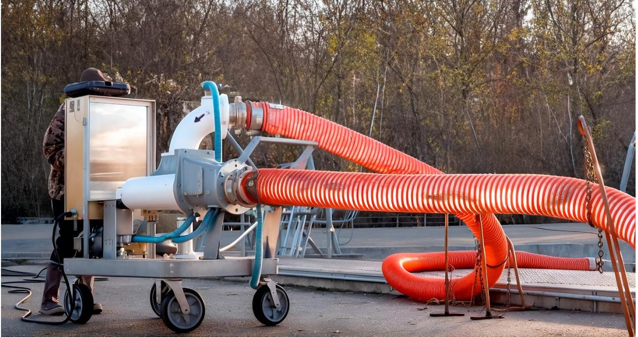
**Figure 143. 'Fish pump', used for mechanised harvesting.**
