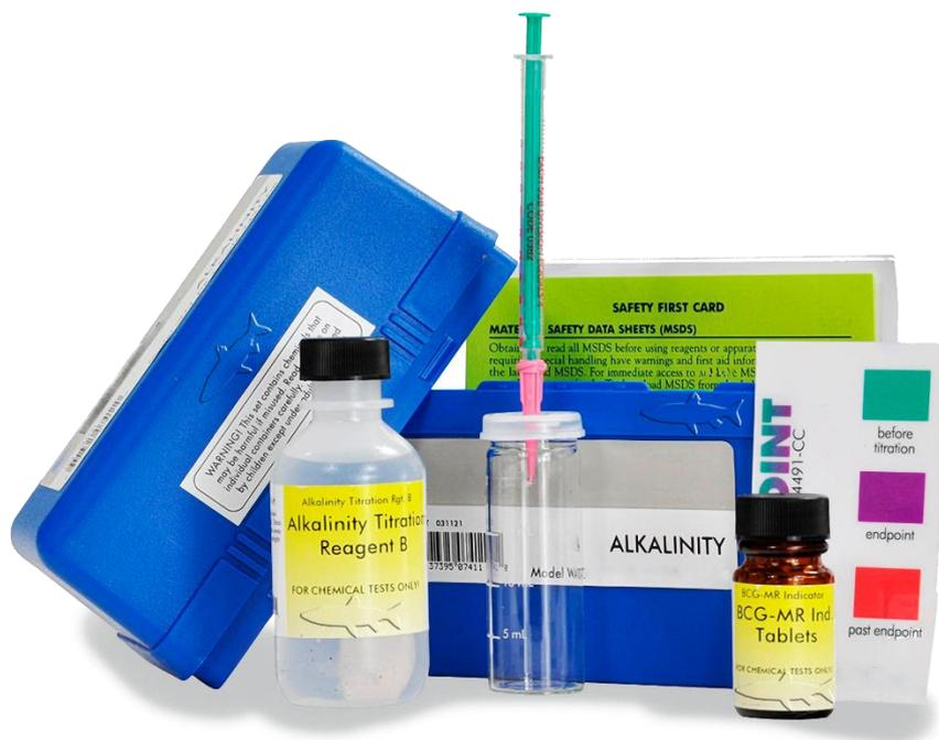
**Figure 48. Titration kit for determining water alkalinity.**
