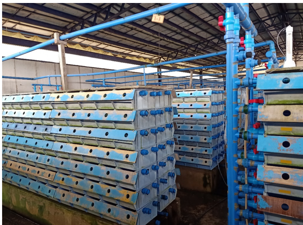
FIGURE 9 Recirculating aquaculture system in vertical “apartments” used for soft-shell crab production
