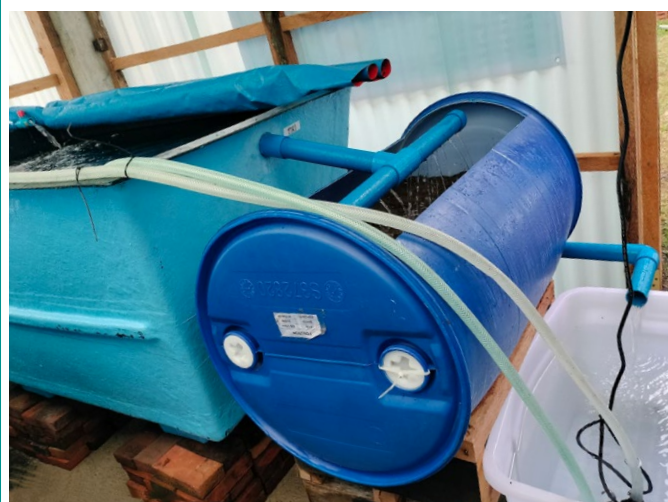
FIGURE 1 Recirculating water system with the use of polychaetae assisted sand biofilters for mud crab broodstock maintenance
