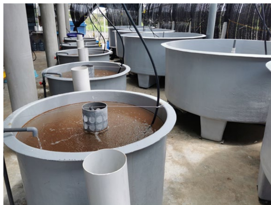
FIGURE 2 Seaweed-based RAS enabled larval rearing tanks
