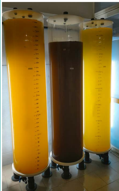
FIGURE 2.8 Algal culture fiberglass cylinders with back lighting
