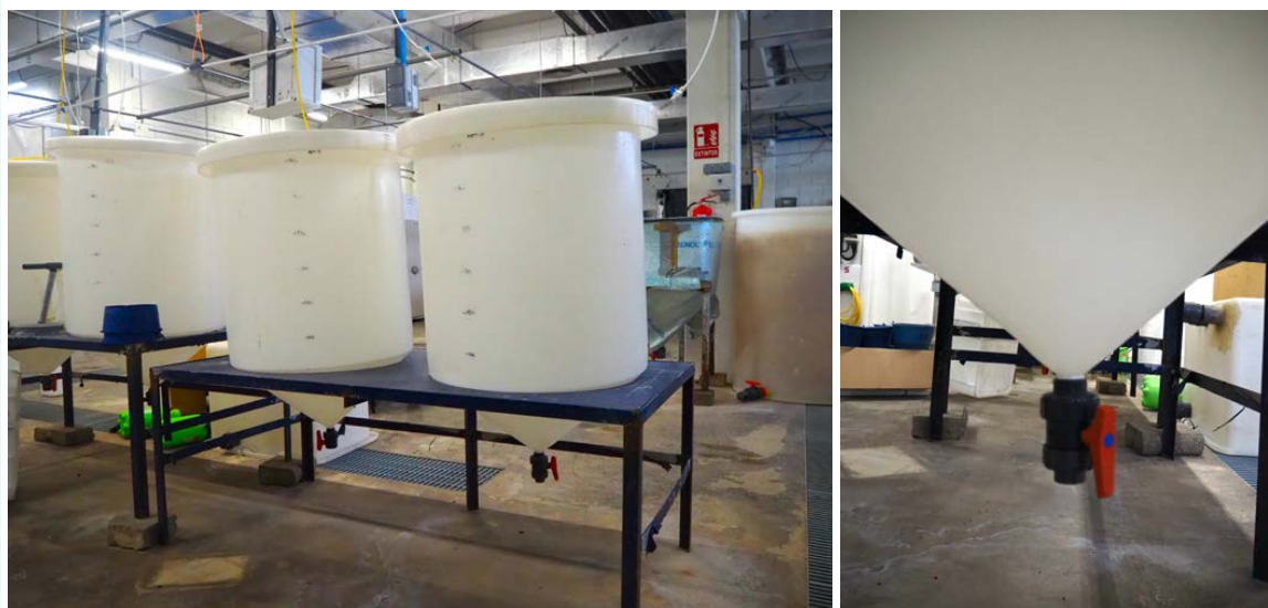
FIGURE 2.10 Rotifer culture tanks that are circular made from plastic that is easily disinfected with a conical bottom and valve for purging and harvesting the rotifers
