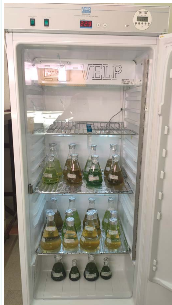
FIGURE 2.6 Stock microalgae culture flasks stored in an incubator
