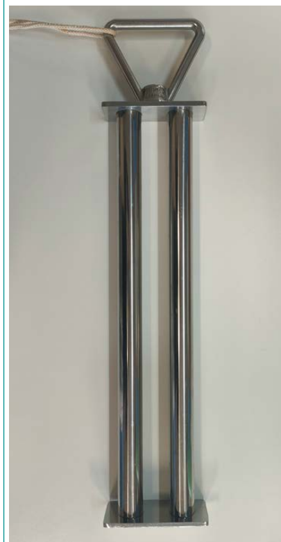
FIGURE 3.12 SEP-Art® separation tool: hatched and unhatched magnetic cysts adhere to the device
