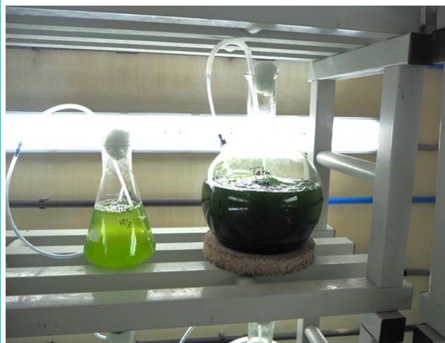
FIGURE 2.5 Algal culture vessels, conical flasks (250–500 ml) and 5–10 L flasks or carboys on shelf with back lighting
