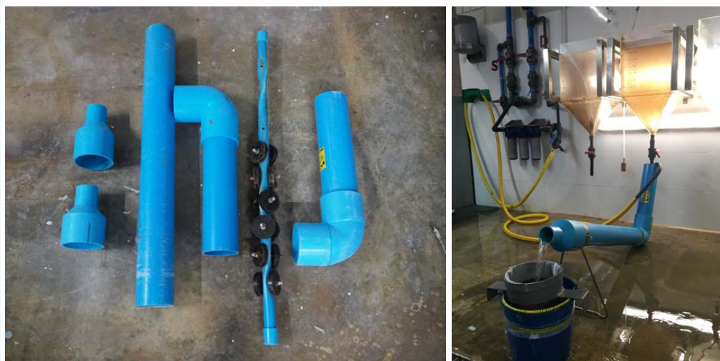
FIGURE 2.12 Artemia harvesting with the PVC SEP-Art® separation tool The inner tube containing circular magnets is inserted into the outer tube (a), which is connected to the tank outlet (b). During tank drainage, unhatched cysts and empty shells are retained on the magnets, while hatched Artemia nauplii pass through the tool and are collected in a mesh bag suspended in a bucket
