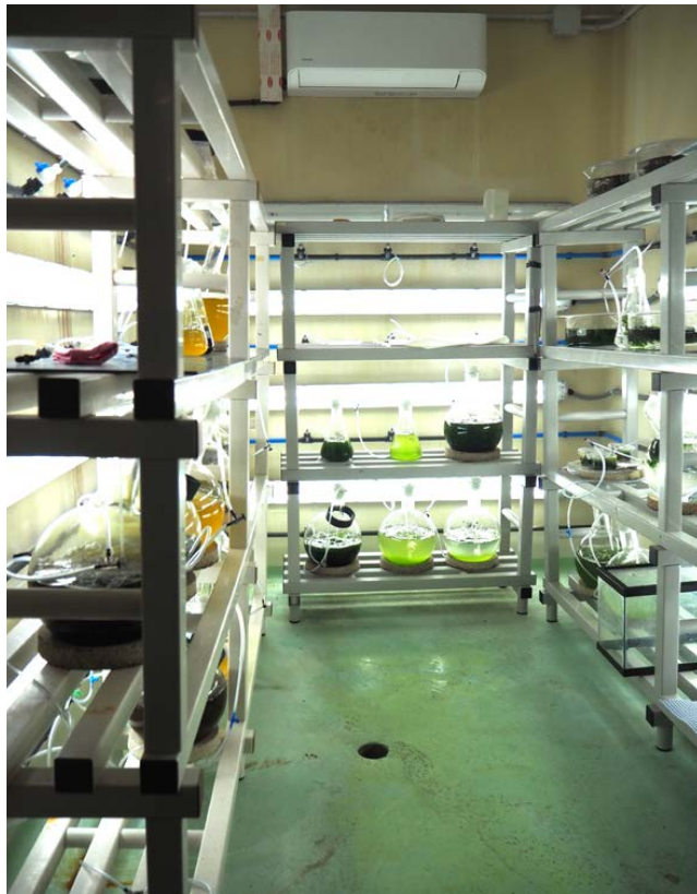
FIGURE 2.4 Pure algal strain room, with controlled environment (air-conditioned), walls and floor that can be disinfected, sloped floor with central drain, shelving with culture vessels and back lighting
