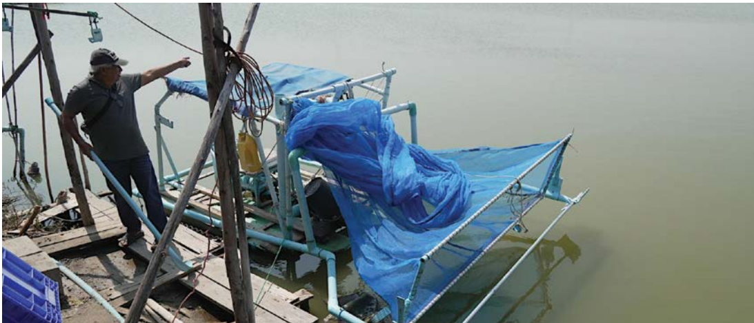
FIGURE 19. Farm-made jet-powered harvesting boat with push net
