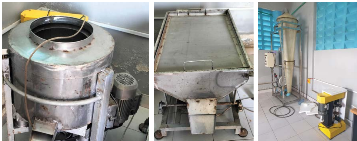
FIGURE 14. From left to right: Centrifuge and a cyst sieve - the Artemia cyst fluidizer and packaging machine, imported by KMFRI from Viet Nam
