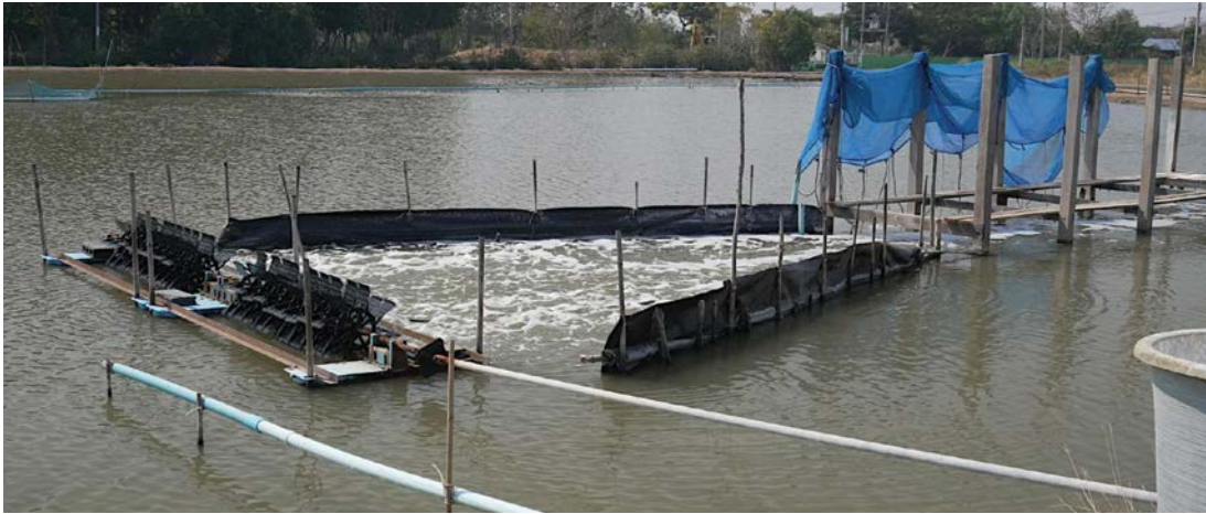
FIGURE 18. Automated biomass harvester directs flow into a net (not deployed)
