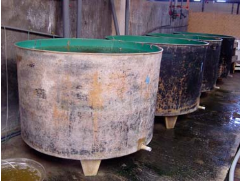
Small fiberglass tanks (1–2 m 3 capacity) for rotifer enrichment.
