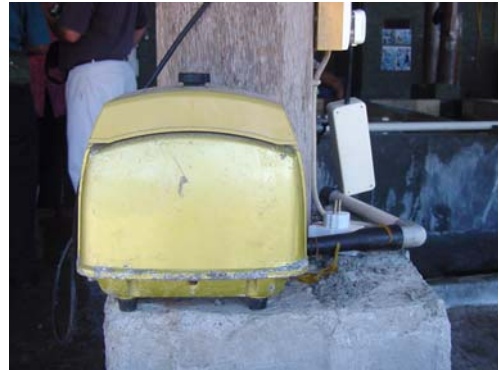
Small air blower used for aeration in small-scale hatchery.
