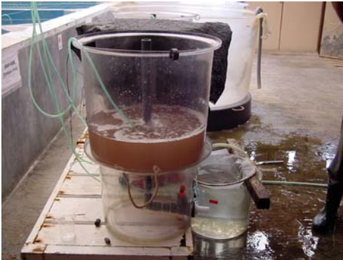
Fiberglass brine shrimp hatching tank, about 50 litres capacity.
