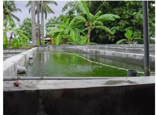
Outdoor microalgal production tanks, about 10 m 3 capacity.
