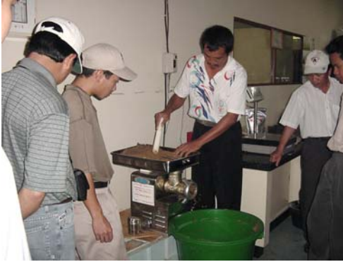
Making moist pellets with a small-scale feed machine.
