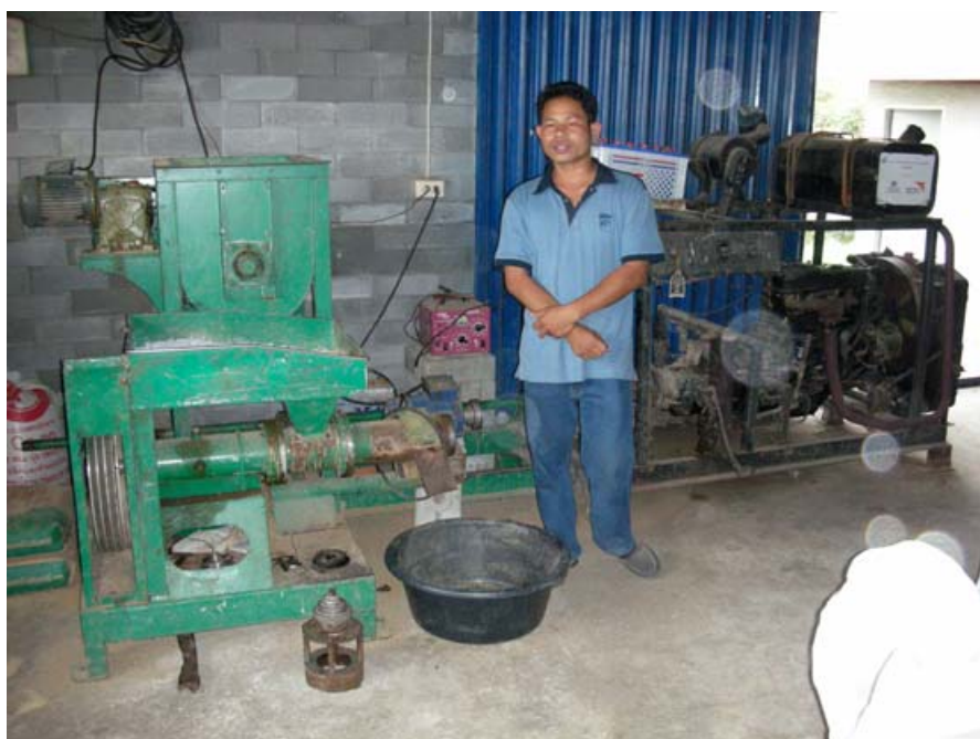
WV staff member demonstrating a small-scale 300 kg/day pelleting machine at the WV Community Centre, Surin.
