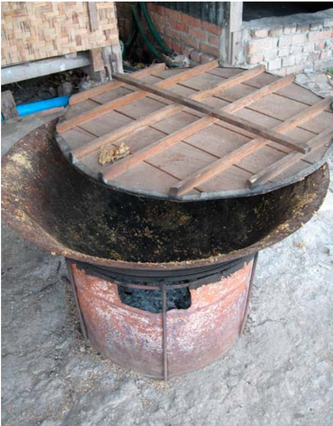
A large wok on top a charcoal stove used to cook feed ingredients.
