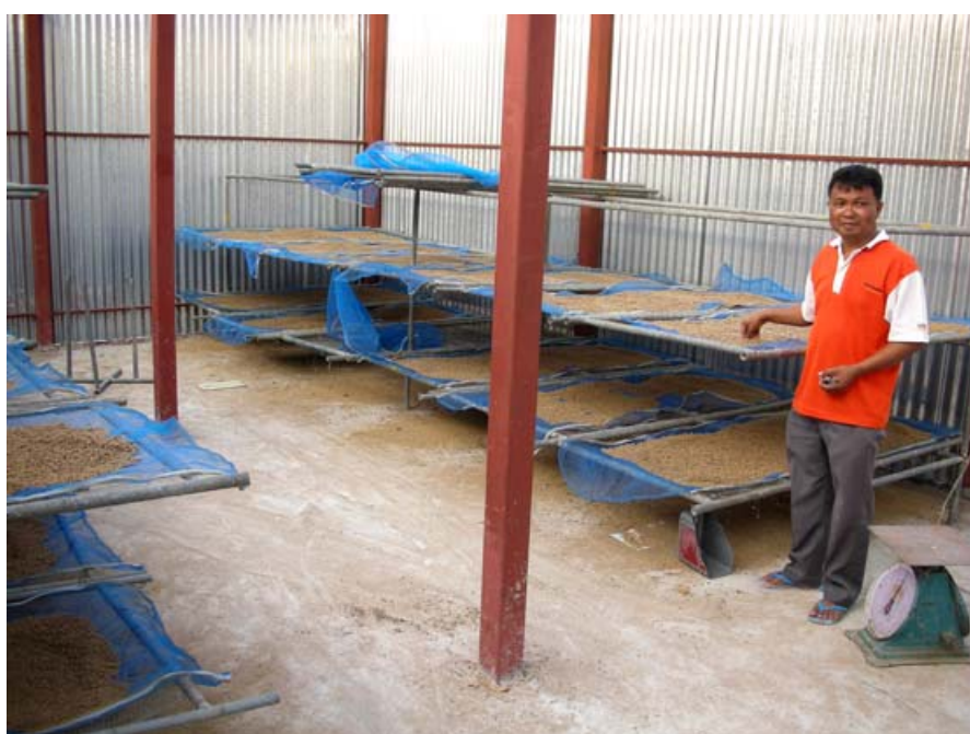
WV staff member inside a small-scale solar pellet drying shed at the WV Community Centre, Surin.
