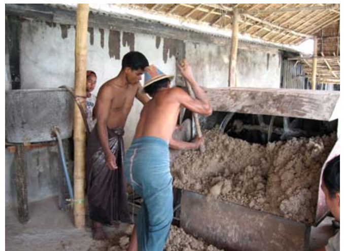
Ingredients are mixed in a large drum mixer for about 5 minutes and fed to fish immediately as a moist mash.
