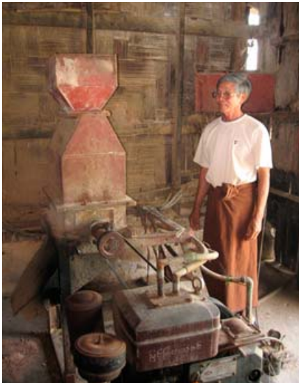
An on-farm grinding machine used to grind dried fish and groundnut cake.
