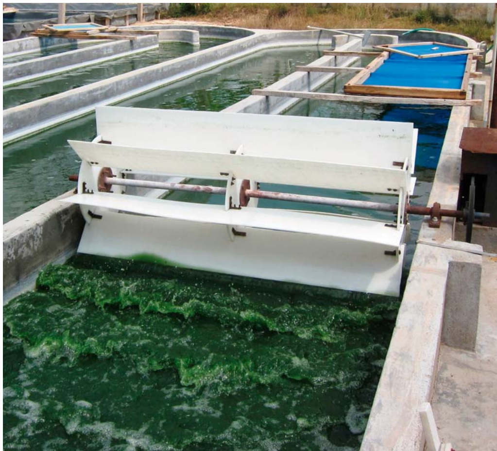
Close up of the paddle wheel and the dense spirulina culture, Nallayan.
