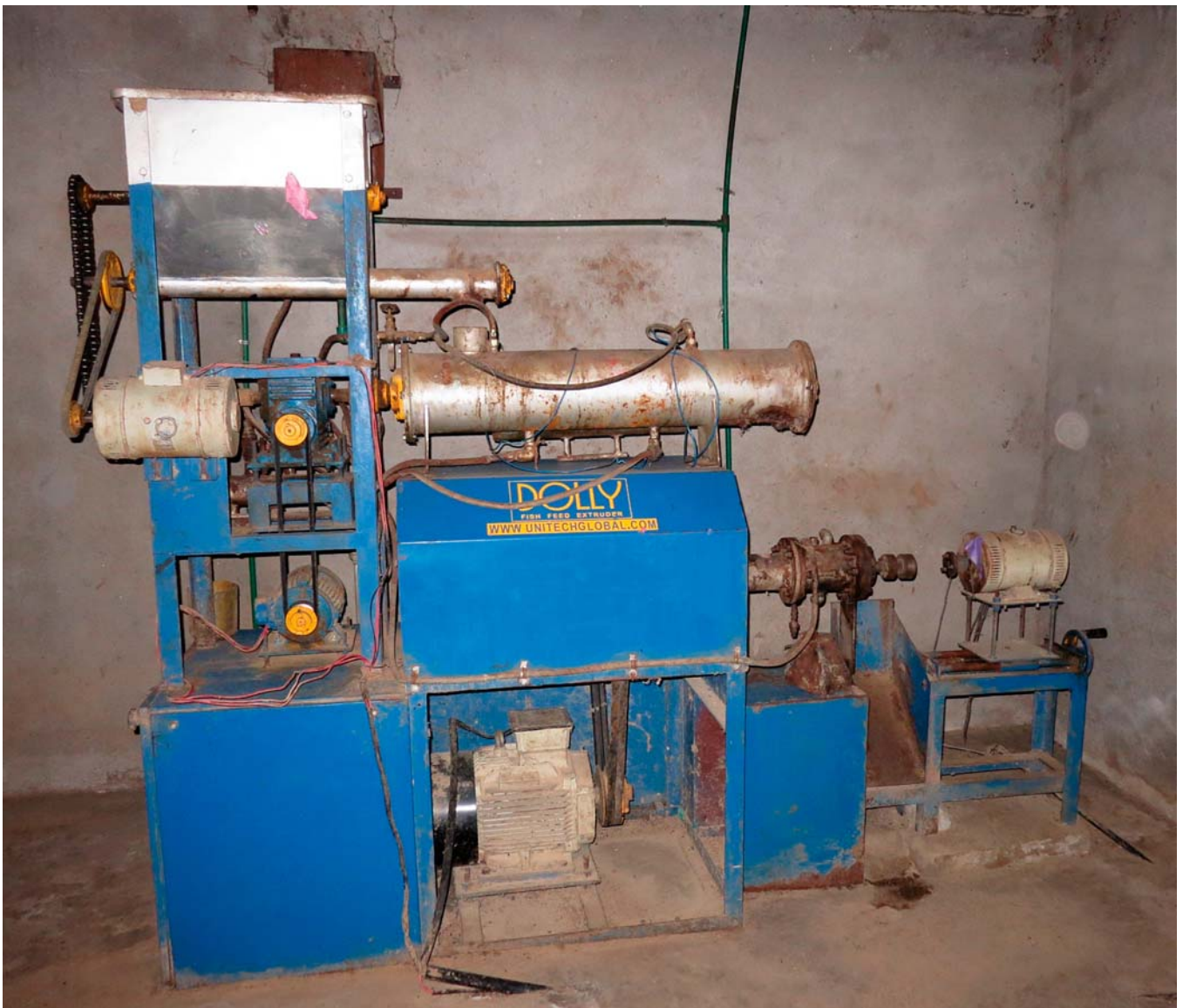
Small-scale Indian extruded pelleting machine, Kathar.
