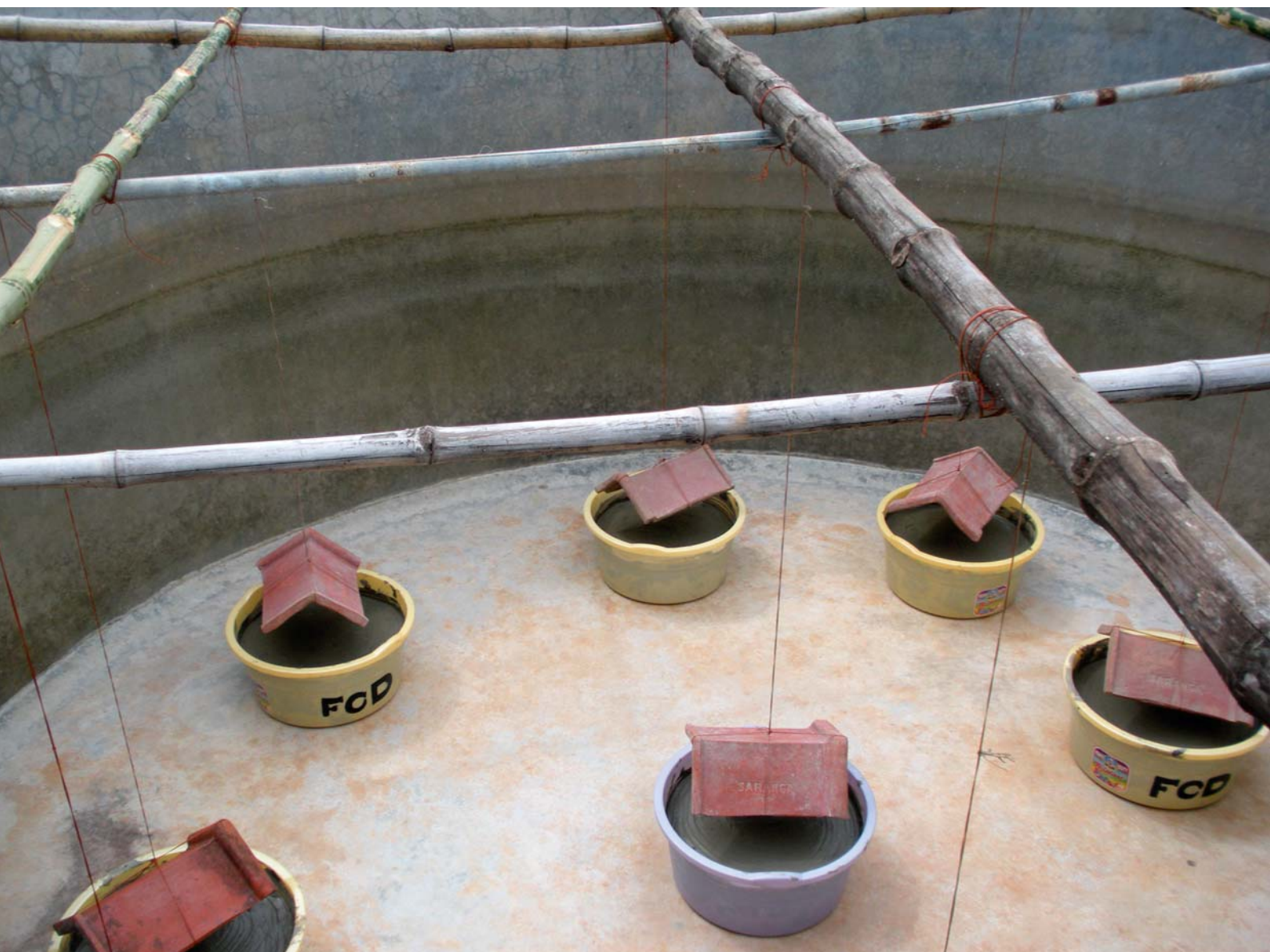
Figure 1: Fired clay tiles served as artificial nesting substrates.
