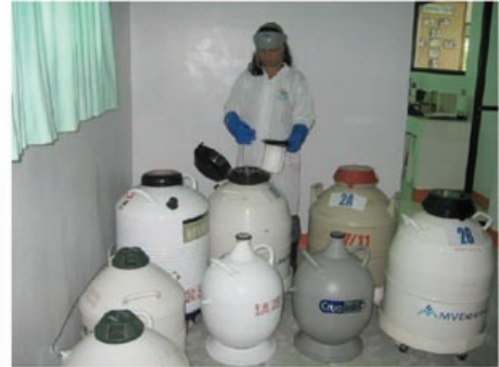
Dewar tanks for keeping cryopreserved tilapia genes
