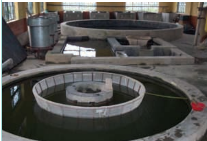
FIGURE 7.20.2 Chinese-style spawning and incubation system
