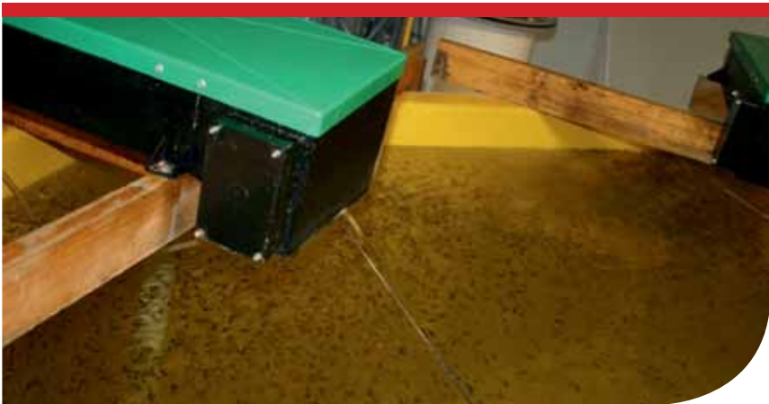
Figure 21 Belt feeder used to wean newly metamorphosed grouper fingerlings (Photo: R. Knuckey)
