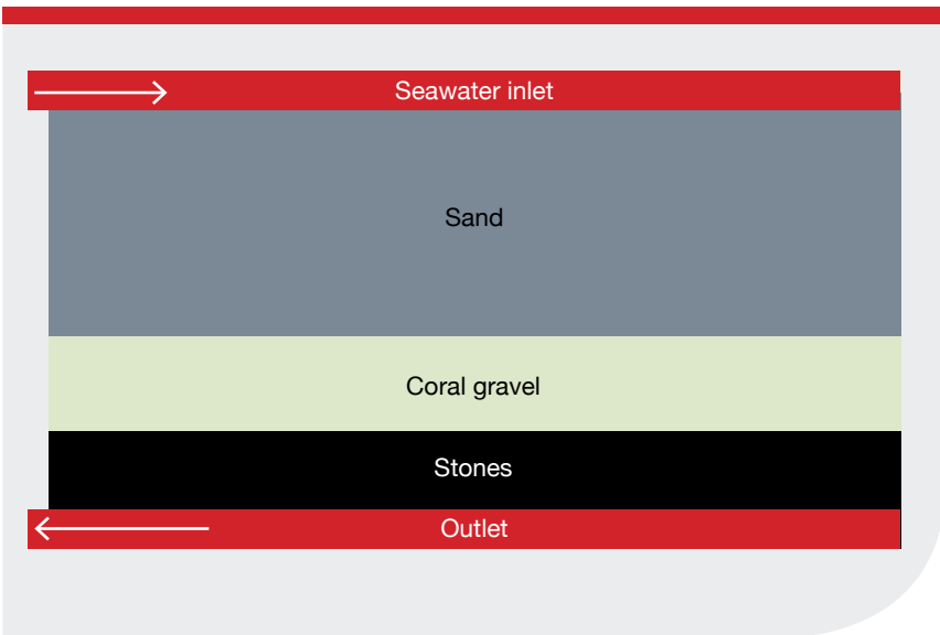
Figure 18 Cross-sectional diagram of a gravity sand filter showing arrangement of graded substrates and inlet and outlet configuration
