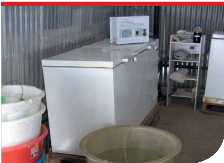
Figure 13 Ozone generator (on top of chest freezer) and seawater tanks set up to wash grouper eggs. The eggs are washed in one tank (foreground), then rinsed in a second tank (out of view). (Photo: M. Rimmer)
