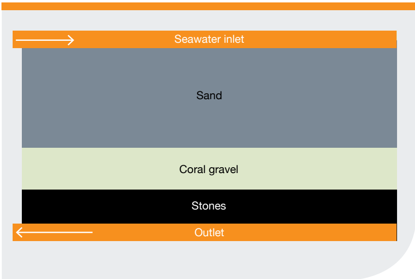
Figure 4 Cross-sectional diagram of a gravity sand filter showing arrangement of graded substrates and inlet and outlet configuration
