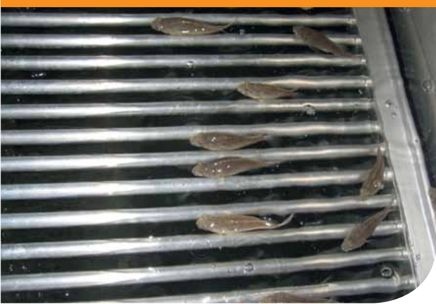
Figure 12 Juvenile (59 days after hatching) tiger grouper ( Epinephelus fuscoguttatus ) being graded using a bar grader, showing how larger fish are retained on the bars—note that the grader works by retaining fish that are wider than the gap between the bars; smaller fish pass through the gaps (Photo: R. Knuckey)
