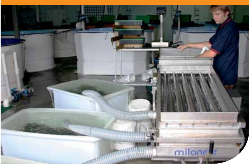
Figure 13 Commercial finfish grader used in Australia to grade tiger grouper. The fingerlings travel down channels that gradually increase in gap width—the fish fall through the gap between the channels and the connecting hoses deliver the fish to separate tanks. Although relatively expensive, commercial graders such as this are capable of grading larger numbers of fish faster than hand-held graders. (Photos: R. Knuckey)
