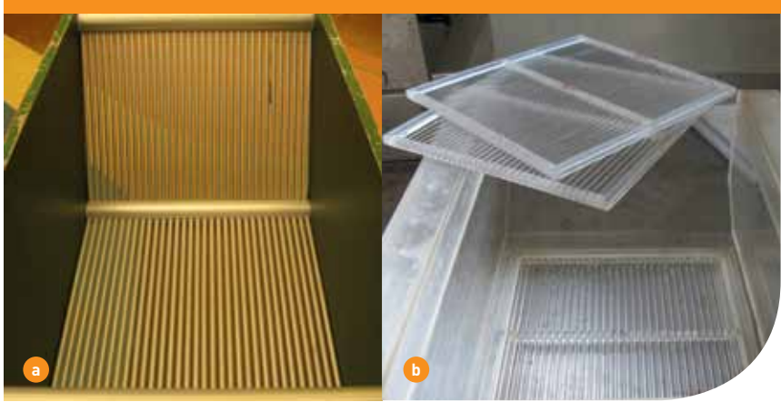
Figure 10 Bar graders: grader (a) has the advantage of having ‘walls’ which allow the grouper to swim actively through the bars, instead of having to lift the grader out of the water to encourage the fish to move through the bars, but the bar width is not adjustable; while (b) has interchangeable panels with different bar widths—the square sections at the sides trap air and provide flotation, enabling the grader to float in the tank (Photos: M. Rimmer)
