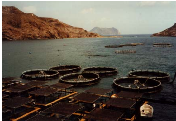
Figure 19: Typical bream farm in Spain using HDPE cage technology and AQ1 feeding system.
