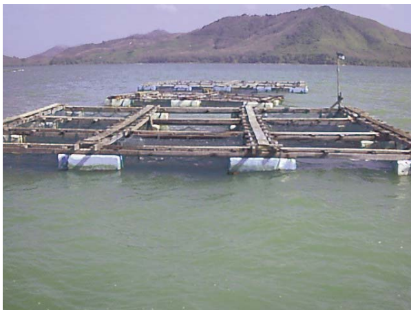
Figure 11: Brood stock wooden sea cage holding facility, Phangnga Coastal Aquaculture Development Centre, Thailand
