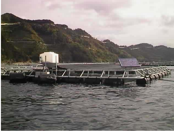
Figure 15: Typical 12x12x10m red sea bream steel cage with AQ1 research feeding system in Japan
