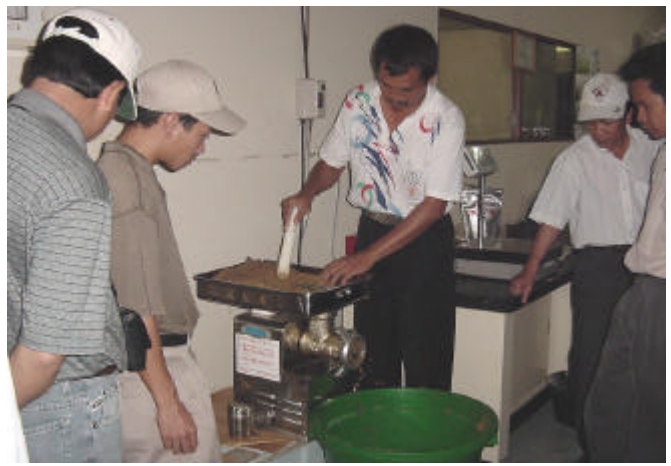
Picture 29: GRIM technician shows participants on how to make pelleted feed by small machine
